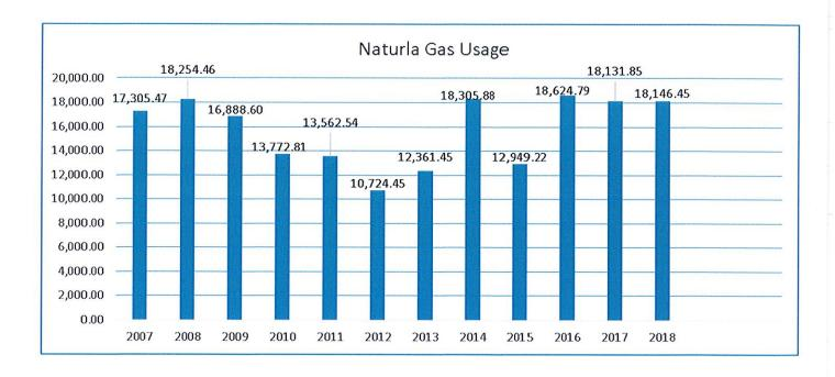
In 2013 we did a heat loss study before doing a major front addition. From that study we made sure to update all new insulation to meet new codes coming in to effect. As well we changed out the 4 main gas furnaces with high efficiency ones.
